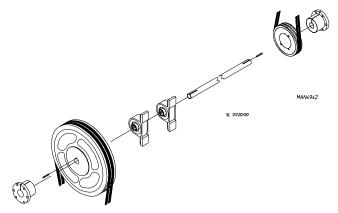
Remove the four bolts holding the two speed reducing shaft pillow block bearings in place and remove shaft assembly from dryer.
